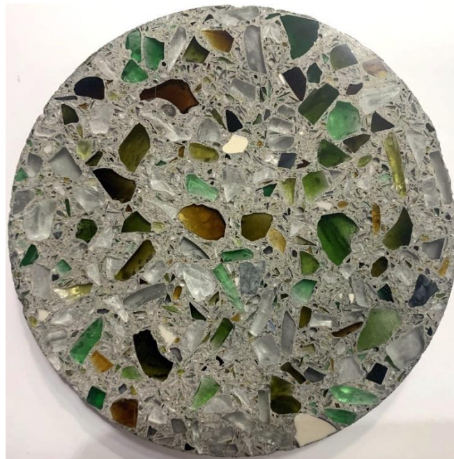
Figure 3.1: A polished disc sample cut from a concrete cylinder made using recycled crushed glass as aggregate. Disc is 100 mm in diameter.
