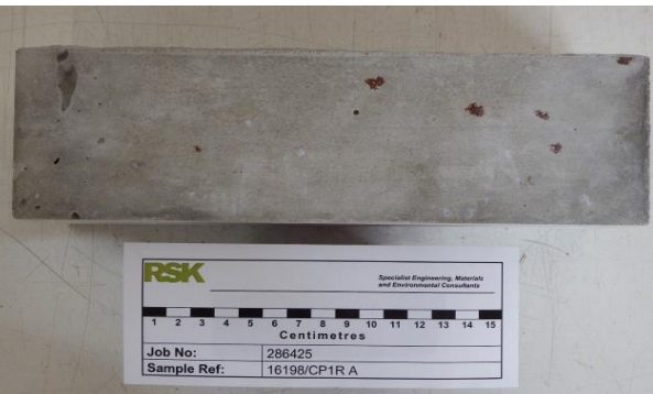
Figure 2.7: Significant reduction in white deposits with the use of GGBS (Mix 4)
