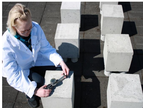
Figure 3.1: Location of measuring studs and measurement of expansion between studs
