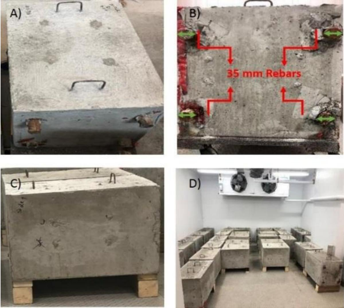
Figure 4.1: Concrete blocks fabricated presenting A) 2D confinement (Top View) B) 2D confinement (Side View) C) 2D confinement (Front View) D) Environmental chamber with 38oC and 100% RH.
