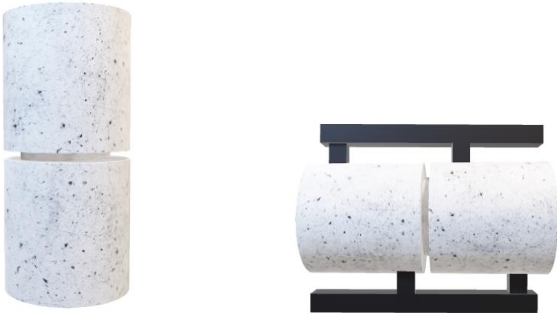
Figure 4.1: Sample with a 22mm notch in the center and the direct shear setup configuration
